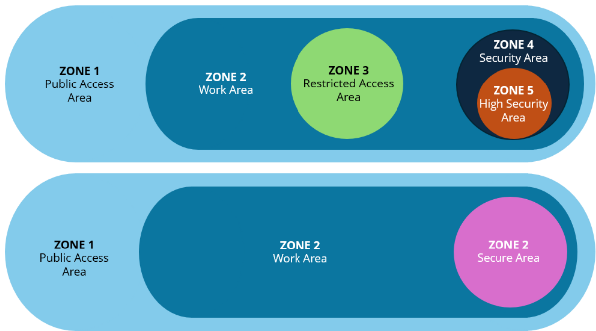
Diagram 1 - Achieving security in depth by layering security zones
